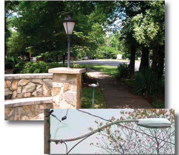
*The lighting at the top is pedestrian-scale lighting, intended to illuminate the sidewalk and adjacent areas. The more conventional street lighting shown on the bottom can also help illuminate the pedestrian areas, but is generally intended to light the travel lanes.*
