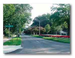
There are a variety of median types. The medians shown above range from minimal to substantial. Functionally, they range from those that simply separate vehicular traffic movements to those that provide fully functional, aesthetic enhancements to the street. The Urban Street Design Guidelines generally discourage minimal, single-function medians.
