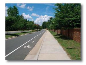
A bike lane in a residential area. The back-of-curb sidewalk is not the preferred treatment, but the bike lane helps to provide a buffer between the pedestrians and motor vehicles.
