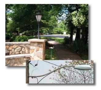
The lighting at the top is pedestrian-scale lighting, intended to illuminate the sidewalk and adjacent areas. The more conventional street lighting shown on the bottom can also help illuminate the pedestrian areas, but is generally intended to light the travel lanes.
