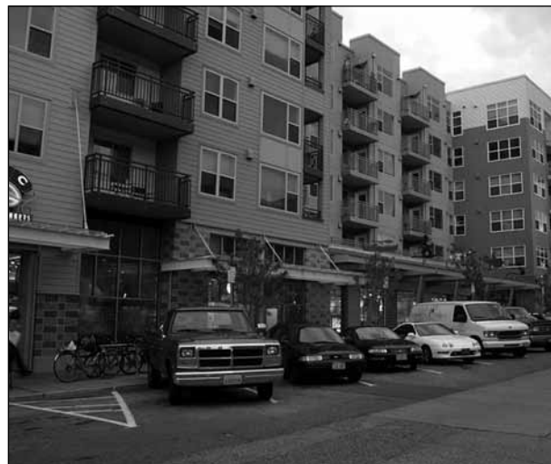
Figure 9.10 Reverse (back-in) angled parking improves driver visibility of bicyclists. Source: Dan Burden, walklive.org.
