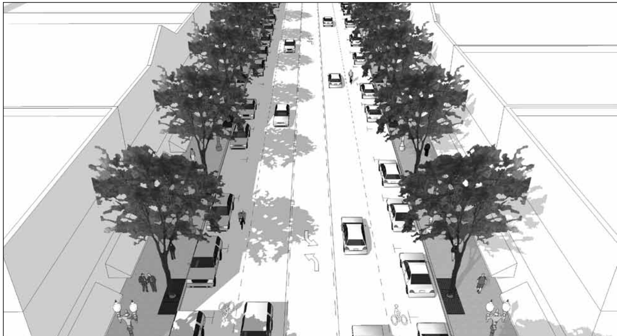
Figure 9.14 Before and after illustration of a road diet. Source: Claire Vlach, Bottomley Design & Planning.
