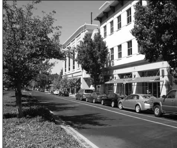
Figure 9.9 A bike lane adjacent to parallel parking on an avenue. Source: Kimley-Horn and Associates, Inc.
