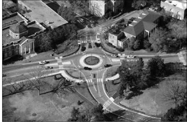
Figure 10.13 Typical layout of a single lane modern roundabout. Source: Kimley-Horn and Associates, Inc.
