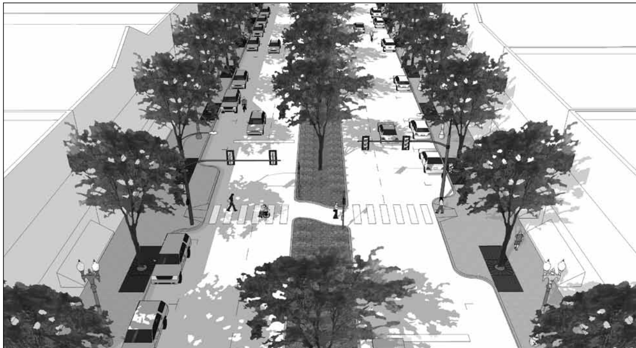
Figure 9.15 Midblock crosswalks provide opportunities to cross streets with long distances between intersection crossings. Source: Claire Vlach, Bottomley Design & Planning.
